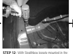
front, use the rear L-bracket mounting hole as a drill guide.
